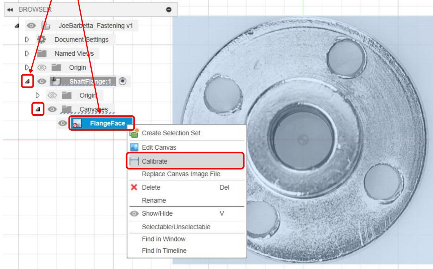
We know the flange diameter is 22 mm from the dimensions given for the part on Amazon.
