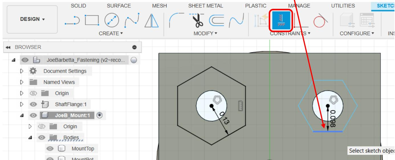
The values of 0.130 and 0.098 were used to create polygons with a width of 0.260" and 0.196". The full size nut for a 4-40 screw has a width of 1/4" (0.250") and the small pattern nut has a width of 3/16" (0.187"). The polygon values will provide some clearance between the walls and the nut sides in the pockets that the nuts will sit in.
