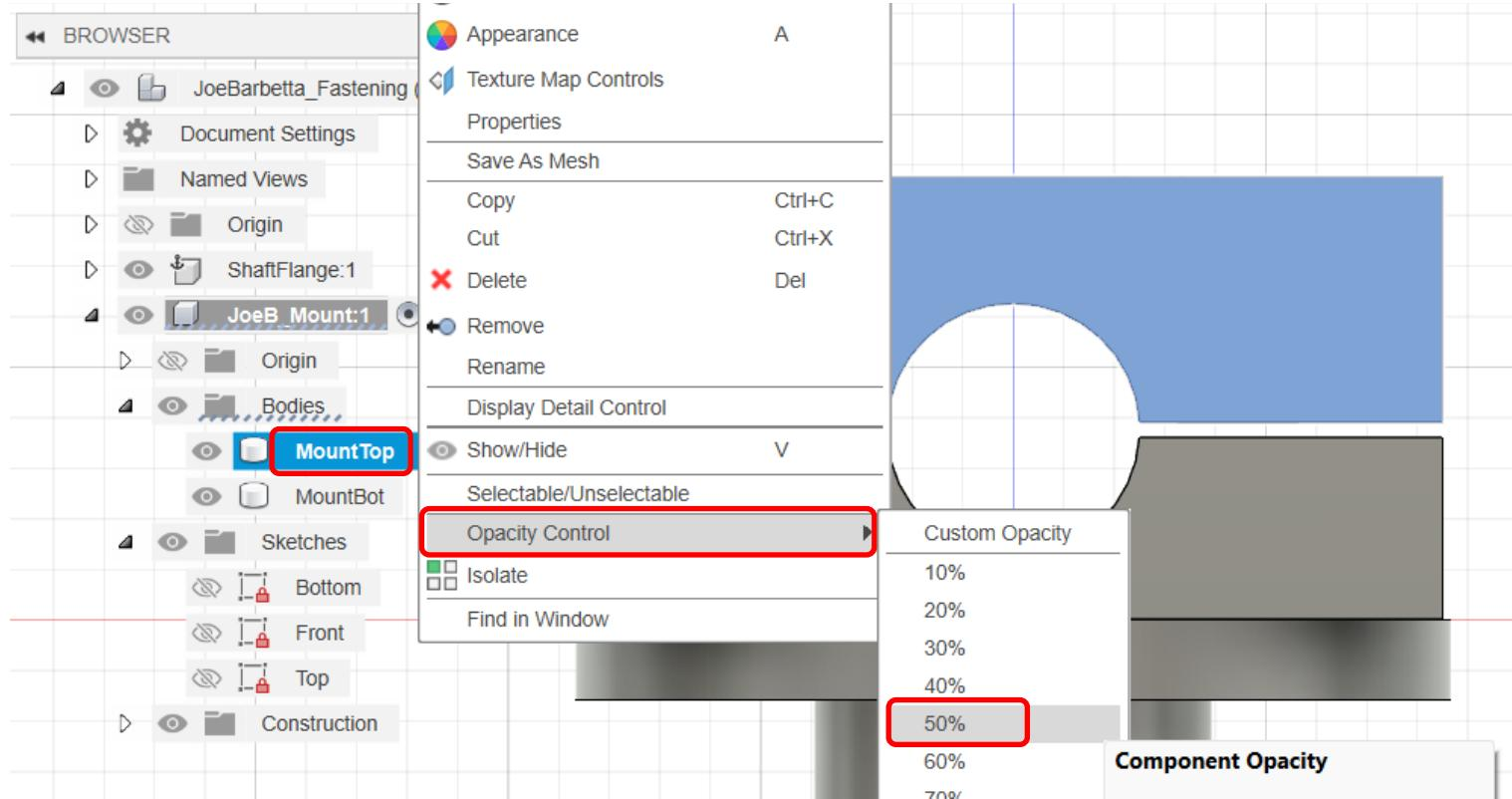
Note how this allows one to see the distance between to bottom edges of the pockets and the horizontal hole for the rod. The pocket depth was chosen so that the 1/2" screws will easily reach the nuts.
