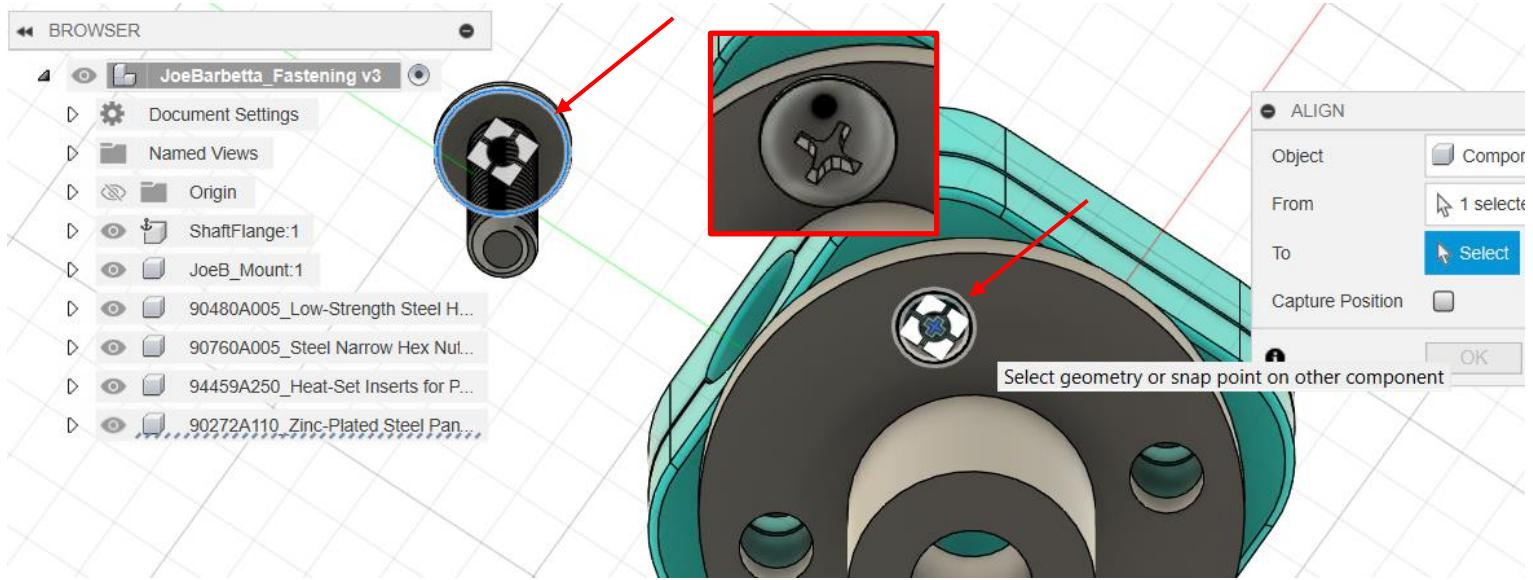
We need 2 more of the screws just inserted. As an alternative to using the import component feature, we will duplicate an already inserted screw.
