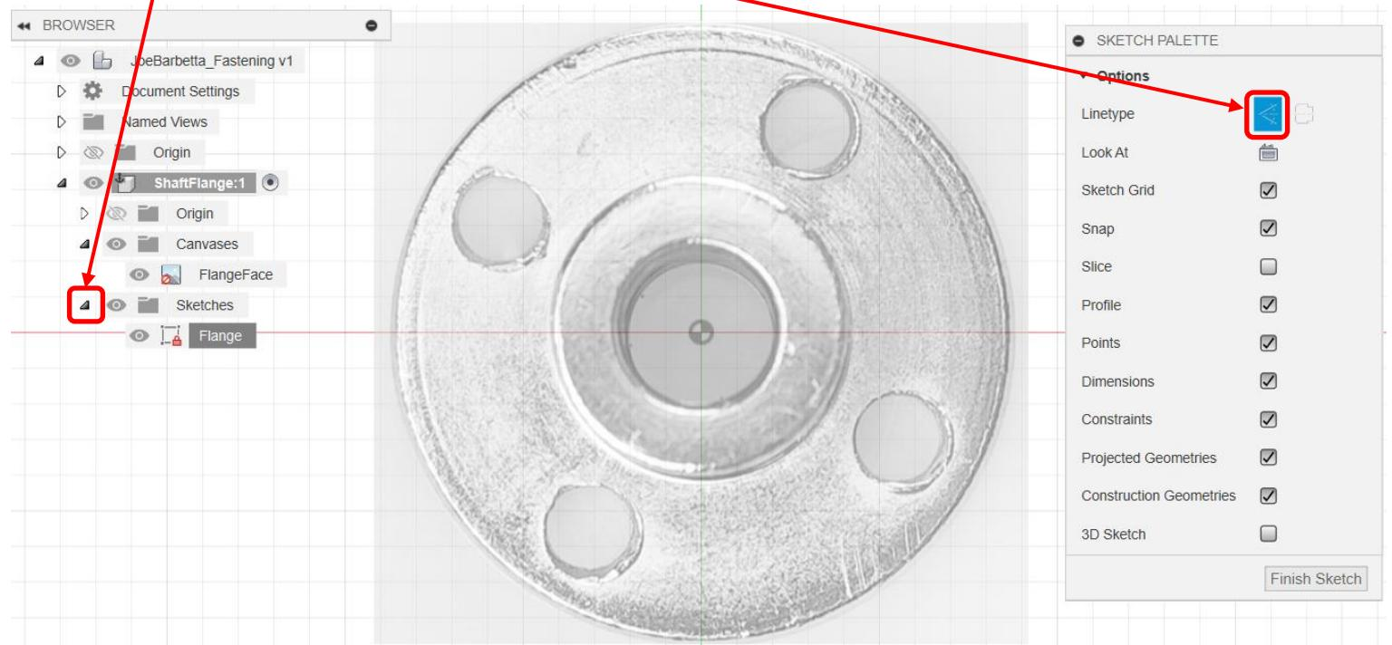
The reason for importing an image of the part is to determine the hole positions, which were missing from the dimensions on the Amazon page. Note that this method can be used to determine dimensions for other parts as well. Nothing beats getting an actual part and measuring sizes and positions with a caliper, but if one wishes to get the design started using an image can serve that purpose. Later on the dimension can be adjusted when the actual part is measured.
