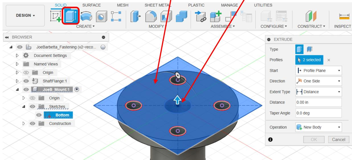
A value of 0.437 will be used for the height of this block. The determination of this value was started by considering that about an 1/8" of material above the 1/4" rod would be adequate to secure the rod and that the material under the rod could be about 1/16" and thus 0.437" (0.125 + 0.25 + 0.062) could be considered for the height of the block.
