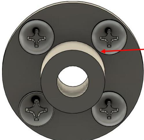
These are common **pan head** screws with a thread size of 4-40. This screw was chosen because it fits nicely in the 3mm (0.118") holes. We could try to a 4-40 screw with a smaller head or choose a slightly longer flat head screw, which would have a smaller head diameter. Ideally, the hole bottoms would be countersunk, but it would work without countersinking the holes. If there is still no room, we could consider a #3 screw.
