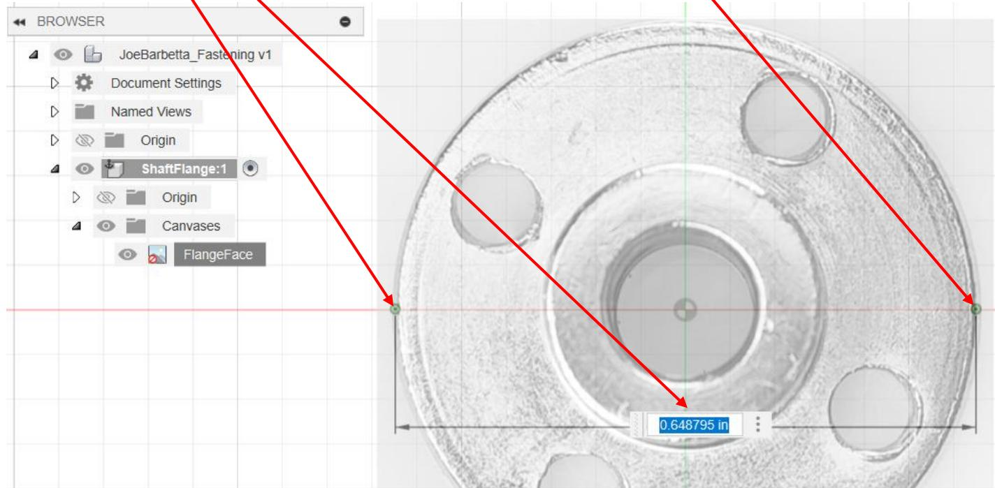
The Canvas image will be scaled so that the 2 point defined will be 22 mm apart and now the image is at a 1 to 1 scale. This will easily allow one to determine the size and/or positions of features.
