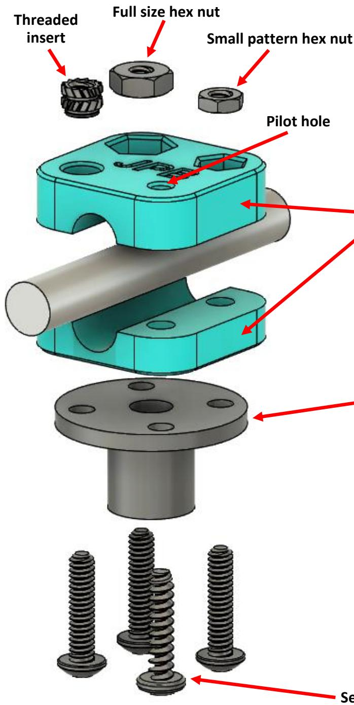
The top mount design demonstrates four different connection methods. Of course one would not employ four different methods in **one part**. One would select the method that is best for a specific application.
