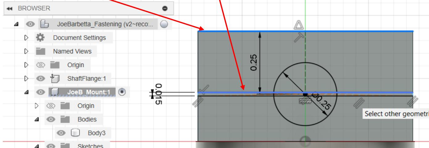
The sketch should look like that below. Note that it is OK if the dimension lines and values are in different locations. Note that the **Front Sketch** shows a **small red lock icon**, which indicates that the sketch is fully constrained.
